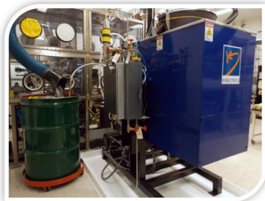
Fukushima's highly alkaline, tritium contaminated water was sent to Canada for desalination using vacuum distillation.
