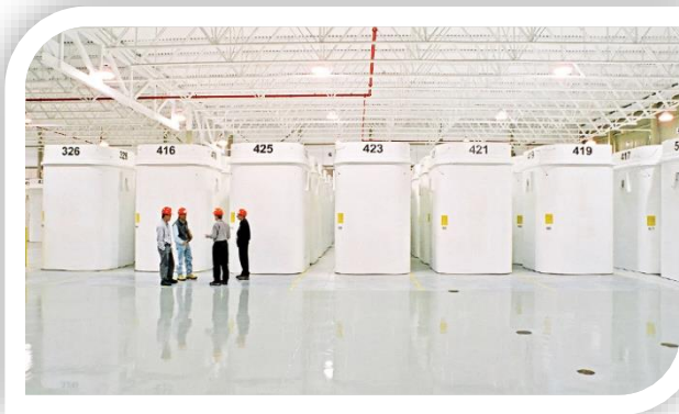
Dry Storage Containers are stored in simple warehouse facilities maintaining a suitable environment for long-term storage.
